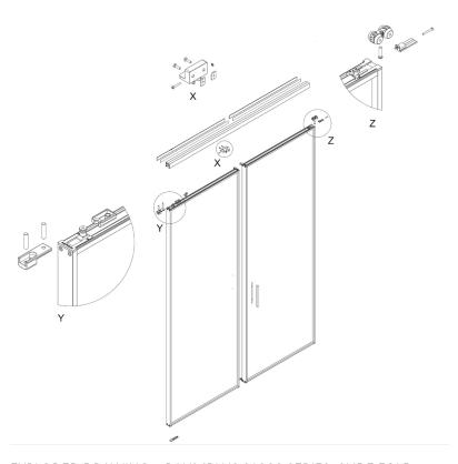
EXPLODED DRAWING – RAUMPLUS S1200 SERIES\_SLIDE FOLD
